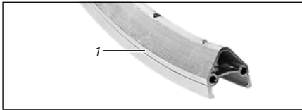
Fig.:60 (Example) 1 Wear indicator
