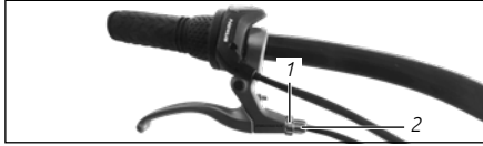
Fig.:45 1 Locknut 2 Knurled nut
