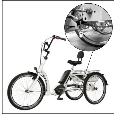
Fig.:51 1 Brake anchor lever
