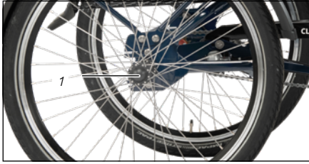
Fig.:59 1 Rear wheel fastening nut
