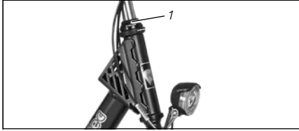
Fig.:30 1 Head tube bearing
