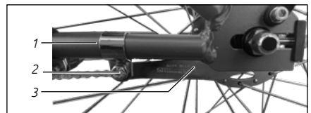
Fig.:48 1 Rear down tube 3 Counterholder
